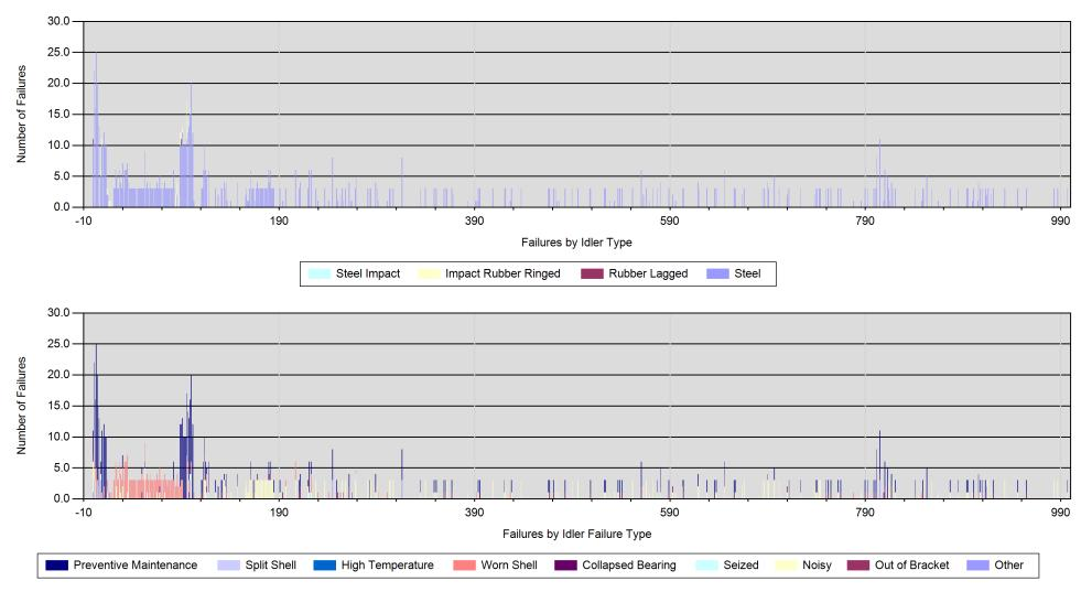
Number of frames on conveyor: 1000 / Total failures during period: 2834
