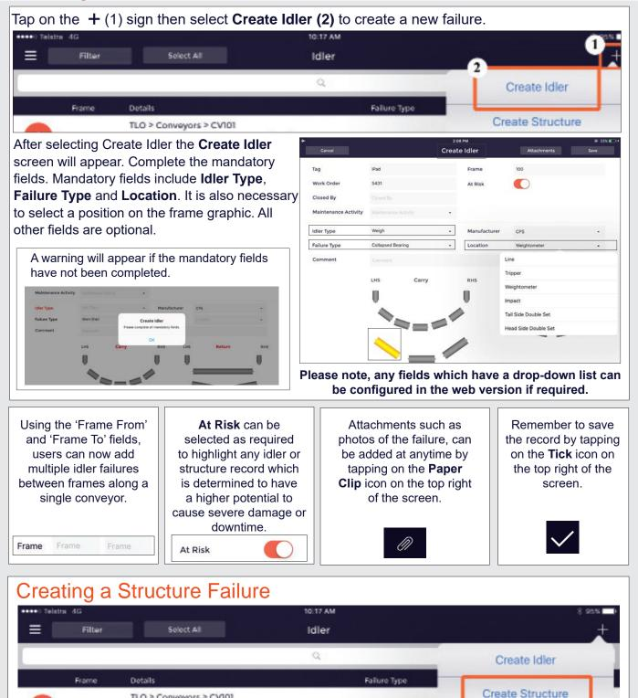
To create a structure failure, follow the same process as creating an idler failure. The save, attachment, voice-to-text functionality is exactly the same. The main difference between creating an idler failure verses a structure failure is that, for a structure failure, the only mandatory fields are Structure Type and Failure Type. All other fields are optional.
